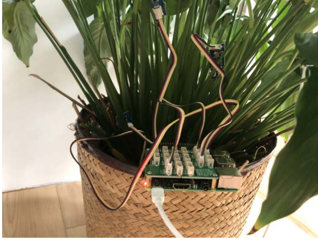
Fig. 2. Indoor plant remote monitoring IoT setup.
